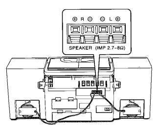
When using the unit with the speakers attached, wind the speaker cables as shown above.
